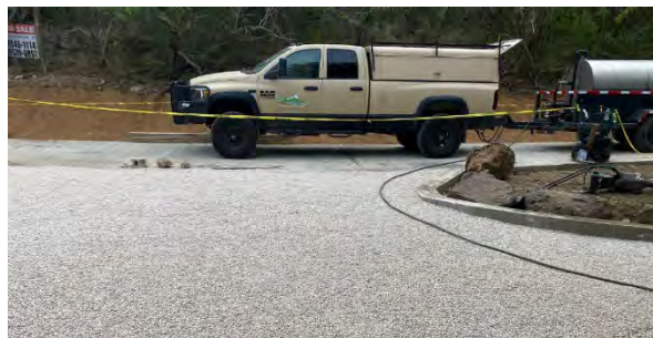
Figure 7. PDC water truck used to irrigate planted trees. While irrigating, PDC personnel also review functionality of the implemented best management practices and apply maintenance as needed
